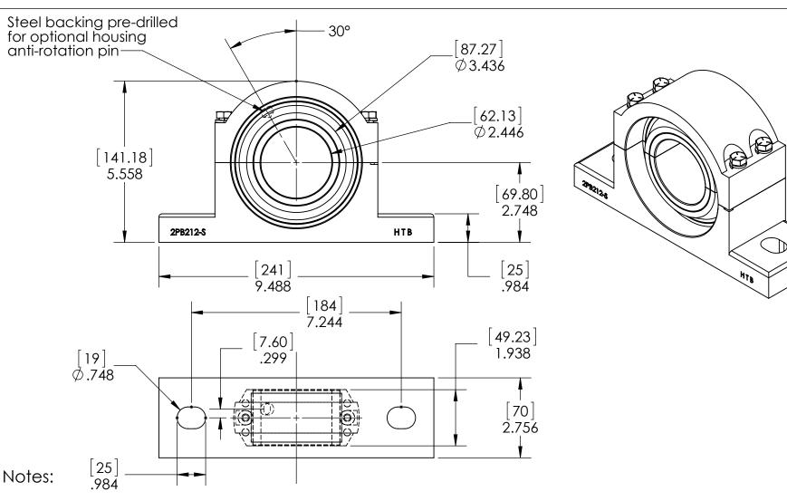
1: When ordering specify sleeve type by adding the suffix HT750, HT100 or NT600 (eg: 2PB212SHT100-244P).
